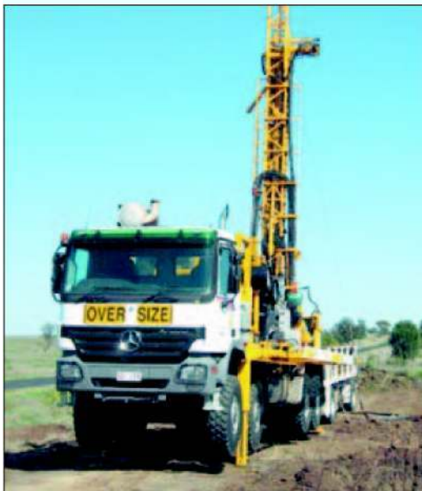
Drilling for coal seam information.
